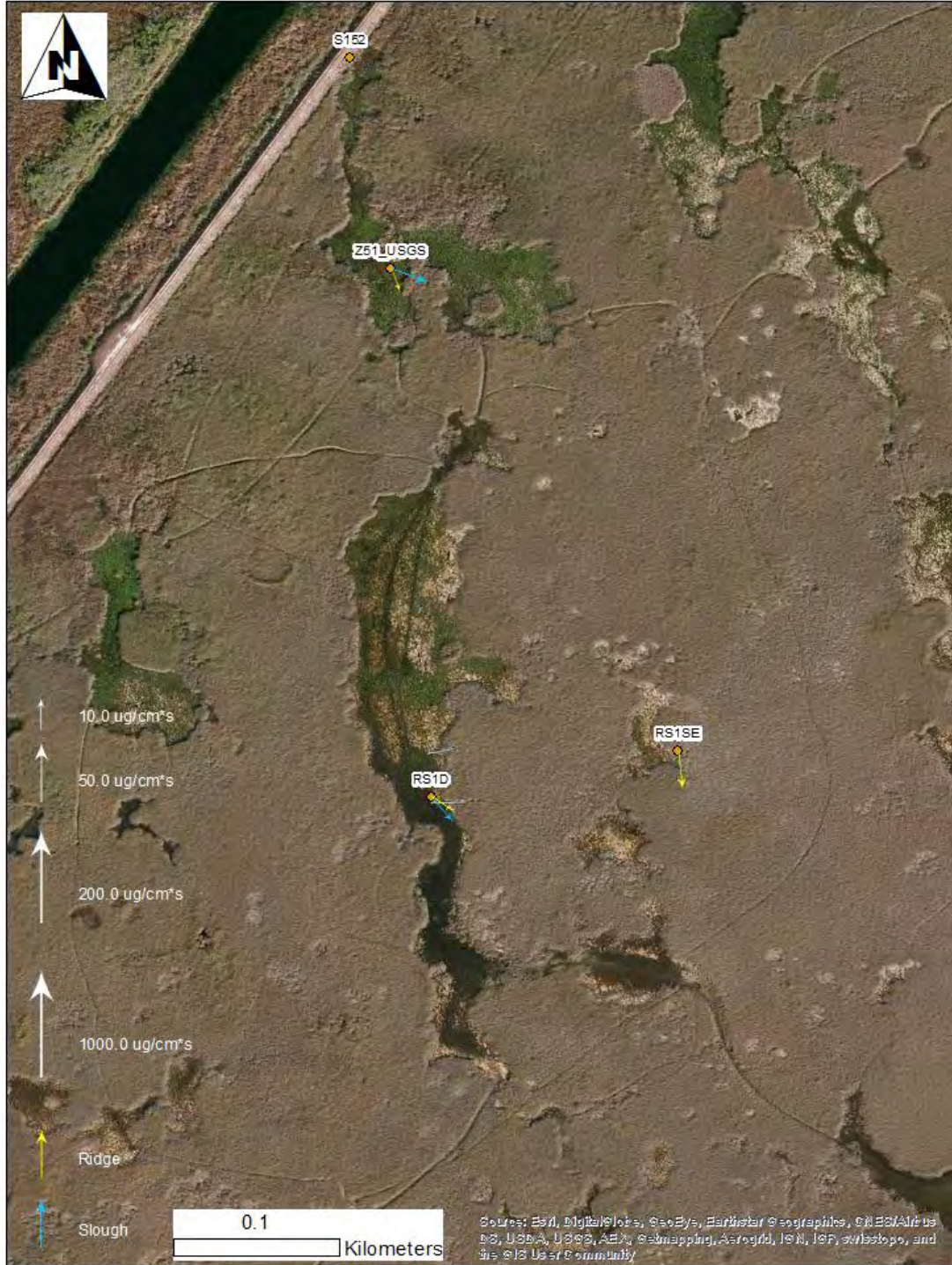
Figure D-190 Post pulse 1 suspended sediment load (during which time the culvert was closed). Samples collected Nov. 19, 2015 at 8:57 at Z51_USGS and 8:45 at RS1D and RS1SE.
