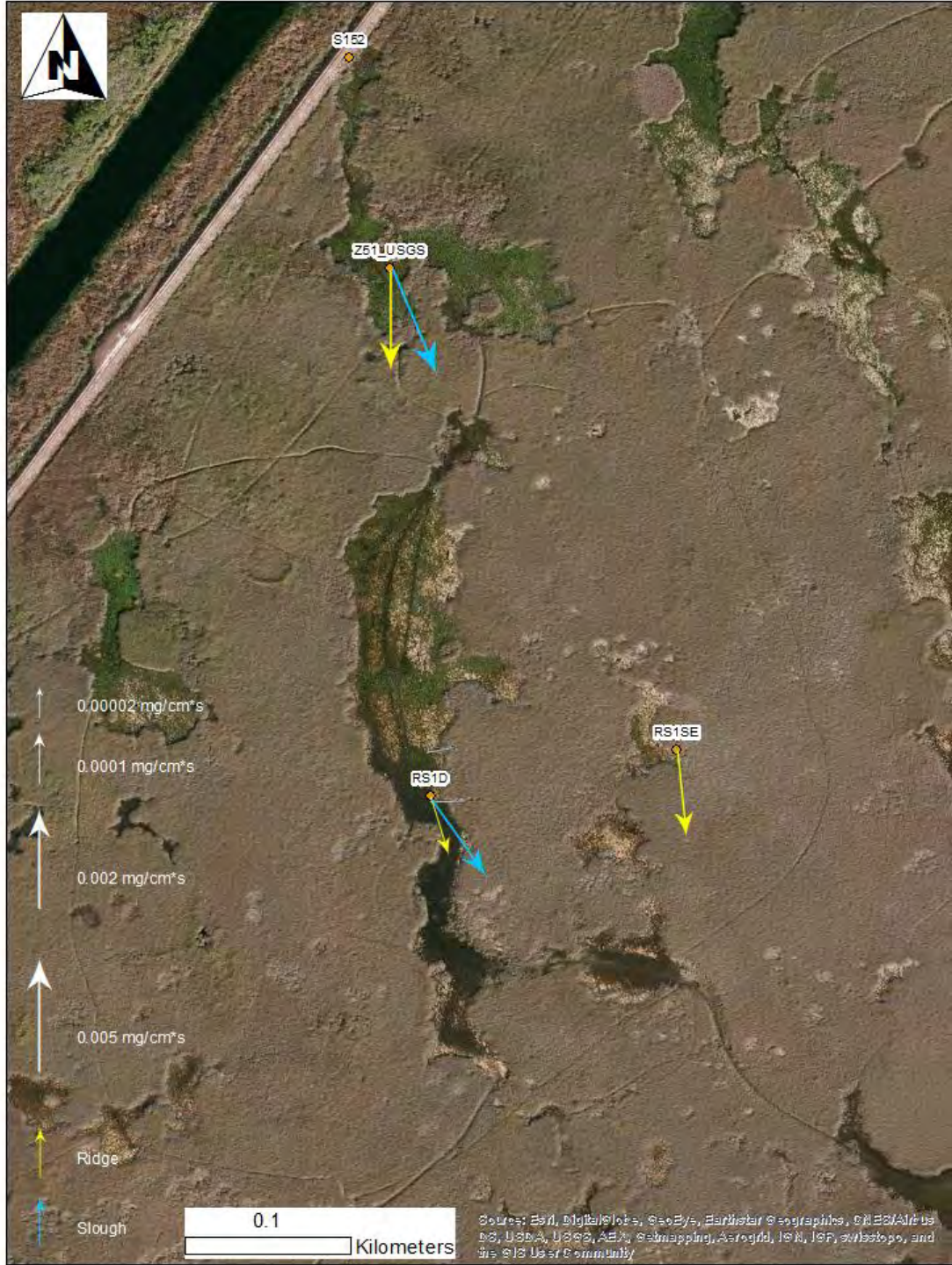
Figure D-206 Transient flow following pulse 2 total phosphorus load. Samples collected Nov. 20 th at 11:06 at Z51_USGS, 8:38 at RS1D and 13:09 at RS1SE.
